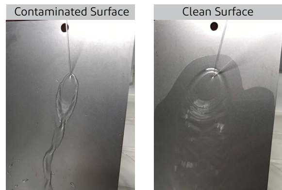
Picture 5: Water-break-free test. Insufficiently cleaned surface (left), well-cleaned surface with water film (right).
